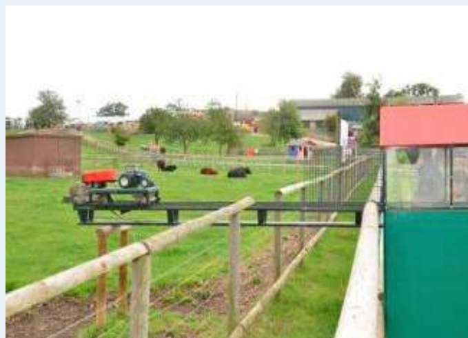
Food is placed in the trailer and by turning a handle the tractor and trailer back out and the food is tipped from the trailer for the cattle
